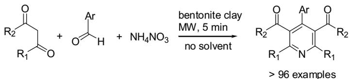
**Scheme 12.23** Microwave-assisted Hantzsch pyridine synthesis.
