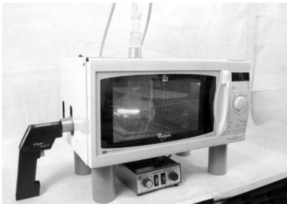
**Fig. 14.6** Photochemistry in a microwave oven (the EDL floats on the liquid surface).
