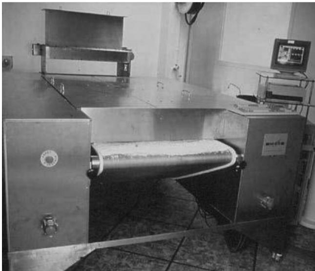
**Fig. 1.18** General view of the Pulsar system. Each applicator is connected to one or two microwave generators set in both side parts of the equipment (courtesy of MES company).
