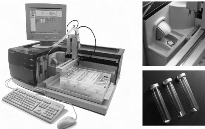
**Fig. 12.6** Monomode microwave reactor with integrated robotics interface for automated use (left). Details of the cavity/gripper (top right) and reaction vials (bottom right) are also displayed (Emrys Synthesizer, Personal Chemistry AB) [86].
