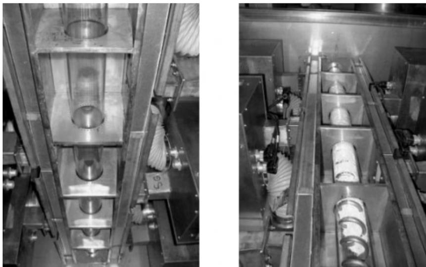
**Fig. 1.19** General view of the Thermostar system. Six successive parallelepiped applicators crossing by a vertical pipe (left) or horizontal pipe with screw (right) (courtesy of MES Company).
