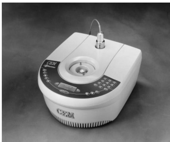
**Figure 12.7** Monomode microwave reactor Discover (without automation) for use with open or sealed vessels of different volumes (CEM Corp.) [81]. A related instrument with automation (Explorer) has recently been introduced.
