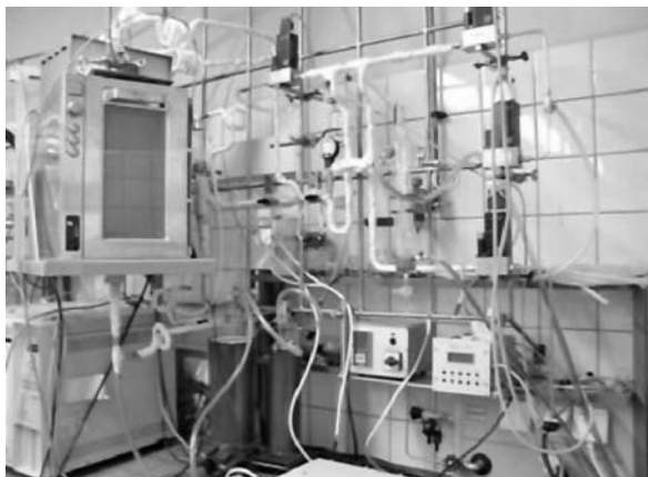
Fig. 2.25. Microwave setup for gas-phase reactions.
