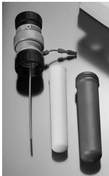
Fig. 16.3. Filtration unit for solid-phase syntheses utilizing the Synthos 3000 (Anton Paar).
