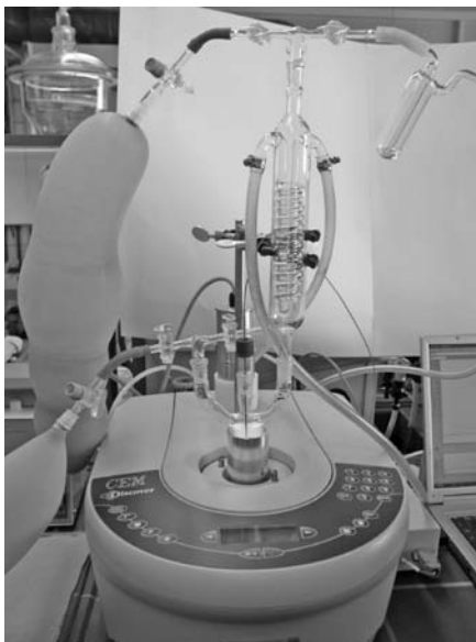
Figure 2.27. Microwave–UV studies based on the Discover™ system.
