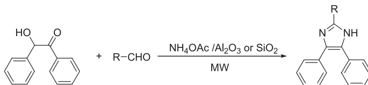
Scheme 8.73. MW synthesis of 2,4,5-substituted imidazolines.
