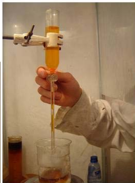
The DCM layer is added to the freebase in an icebath, the freebase is first dissolved in the same volume of glacial acetic acid.
