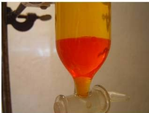
The DCM phase absorbing the bromine.
