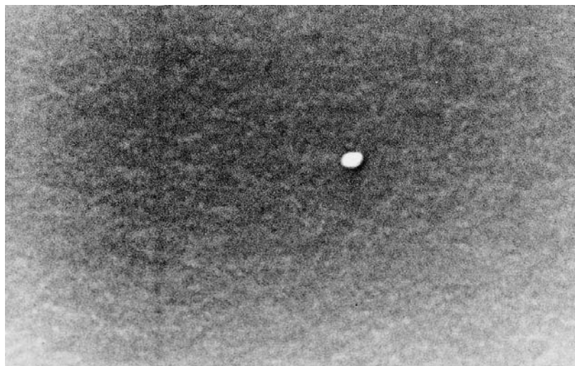
Figure 5 Scanning electron micrograph of the internal surface of a gel resin. Magnification \times 17000 . (University of Manchester Electron Microscopy Unit, courtesy of Hoechst Celanese Corporation.)
