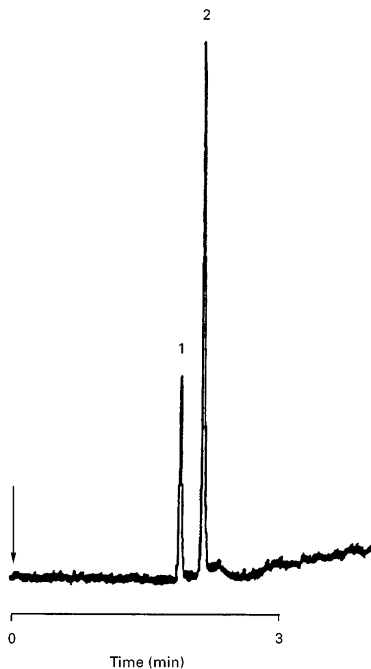
Figure 12 Volatile sulfur impurities in propylene on a silica PLOT column. Experimental details: column, 30 m \times 0.32 mm fused silica CP-SilicaPLOT, d_f = 4 \mu\text{m} ; oven, 50°C \rightarrow 120°C, 10°C \text{min}^{-1} ; carrier gas, helium; injection, valve, 375 \mu\text{L} propylene; detection, sulfur chemiluminescence detection. Peaks: 1, carbonyl sulfide (34 p.p.b.); 2, hydrogen sulfide (108 p.p.b.).
