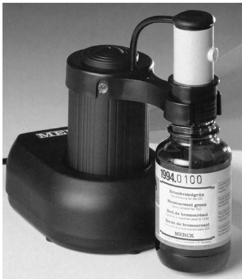
Figure 2 (See Colour Plate 33) An electropneumatically operated spray system for TLC. (Reproduced with the permission of Merck Ltd., UK.)
