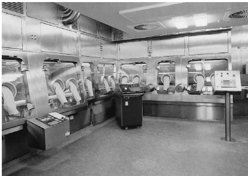
Figure 13 (See Colour Plate 37). Isolator, Class 100, for filling, transportation and loading of vials into the freeze-drying plant. Decontamination of the isolator and the equipment therein is accomplished by vaporized hydrogen peroxide (VHP). The VHP 100® generator can be seen in the centre in front of the isolator. (Courtesy of Steris GmbH, Hürth, Germany.)
