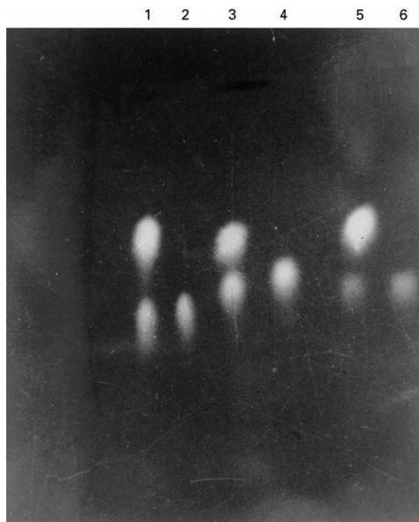
Figure 2 Chromatogram showing resolution of Dns-DL-phenylalanine, valine and leucine. From left to right: 1, Dns-DL-phenylalanine; 2, Dns-L-phenylalanine; 3, Dns-DL-valine; 4, Dns-L-valine; 5, Dns-DL-leucine; 6, Dns-L-leucine. Developing solvent, aq. 0.5 mol L -1 sodium chloride + acetonitrile (15 + 1). Developing time 20–25 min. Detection 254 nm.
