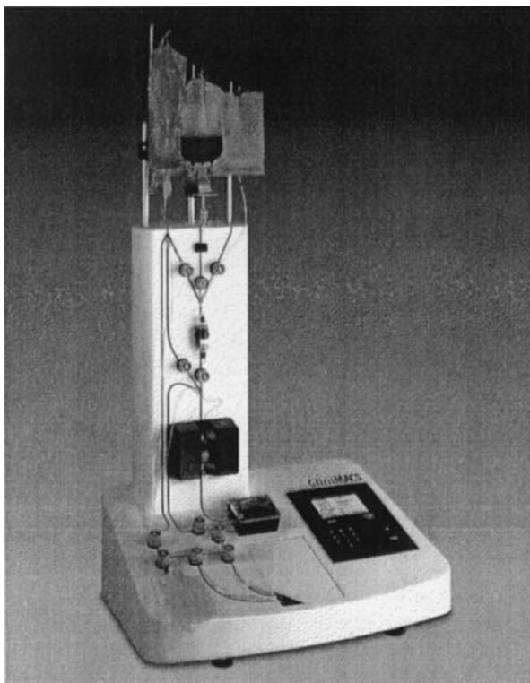
Figure 3 (See Colour Plate 65). Computer-controlled magnetic cell sorter CliniMACS. Courtesy of Miltenyi Biotec, Bergisch Gladbach, Germany.
