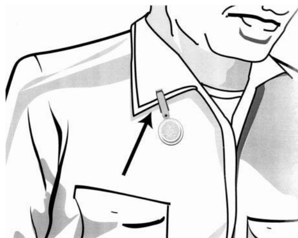
Figure 3 Diffusive sampler attached to a worker. This method is more acceptable to workers but the uptake rate varies from chemical to chemical and cannot be altered by field hygienists.
