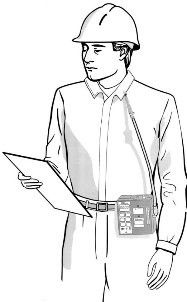
Figure 2 Personal air sampling train attached to a worker.
