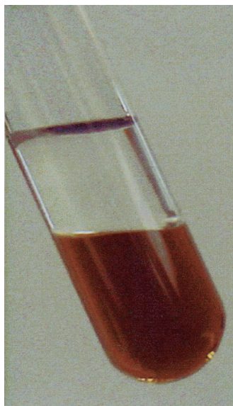
Figure 1. Two-phase system consisting of (top phase) toluene and (bottom phase) perfluoro-2-butyltetrahydrofuran (Fluoroinert FC-75). The dark color (brown) in the bottom phase indicates that the dendrimer-encapsulated Pd nanoparticles, complexed with poly(hexafluoropropylene oxide- co -difluoromethylene oxide) monocarboxylic acid, are selectively extracted into the fluoruous phase. No detectable color was observed in the organic phase.
