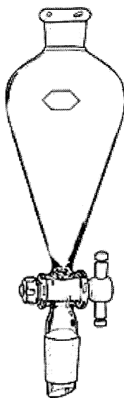
Figure 010. A standard laboratory separatory funnel.
