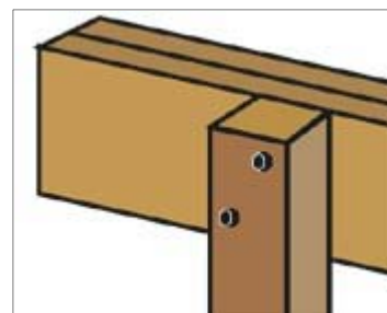
Image E: For a sturdy beam, secure posts to beams with offset carriage bolts. Notice the 12 3/4" overhang.
