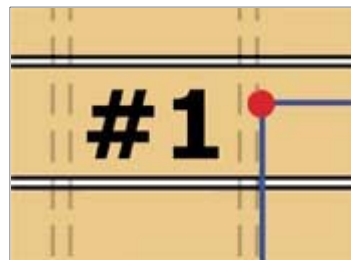
Image B: Notice here that the deck joist is located on the outside edge of the mark. ( Click here for top view )
