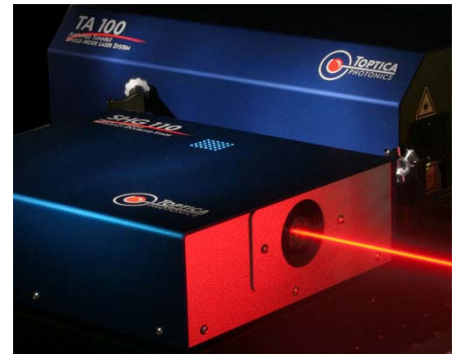
Fig. 16: TOPTICA's DL-SHG 110 module: by locking the resonator of the SHG 110 module to the diode laser, and therefore resonantly enhancing the fundamental light, 5 mW @ 614 nm could be generated from 12 mW @ 1028 nm.
