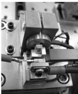
Fig. 3. Prototype for the eyesafe microchip laser.
