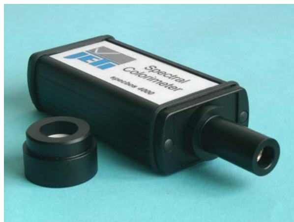
Fig. 8 Colorimeter specbos 4000 with calibration standard
