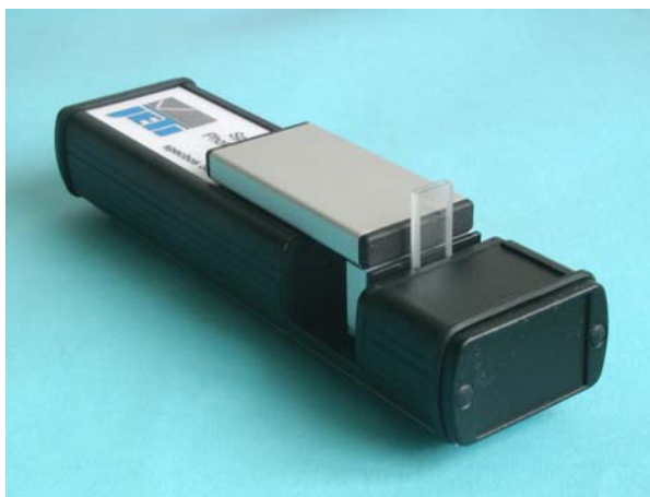
Fig. 9 Spectral photometer specbos 3000
