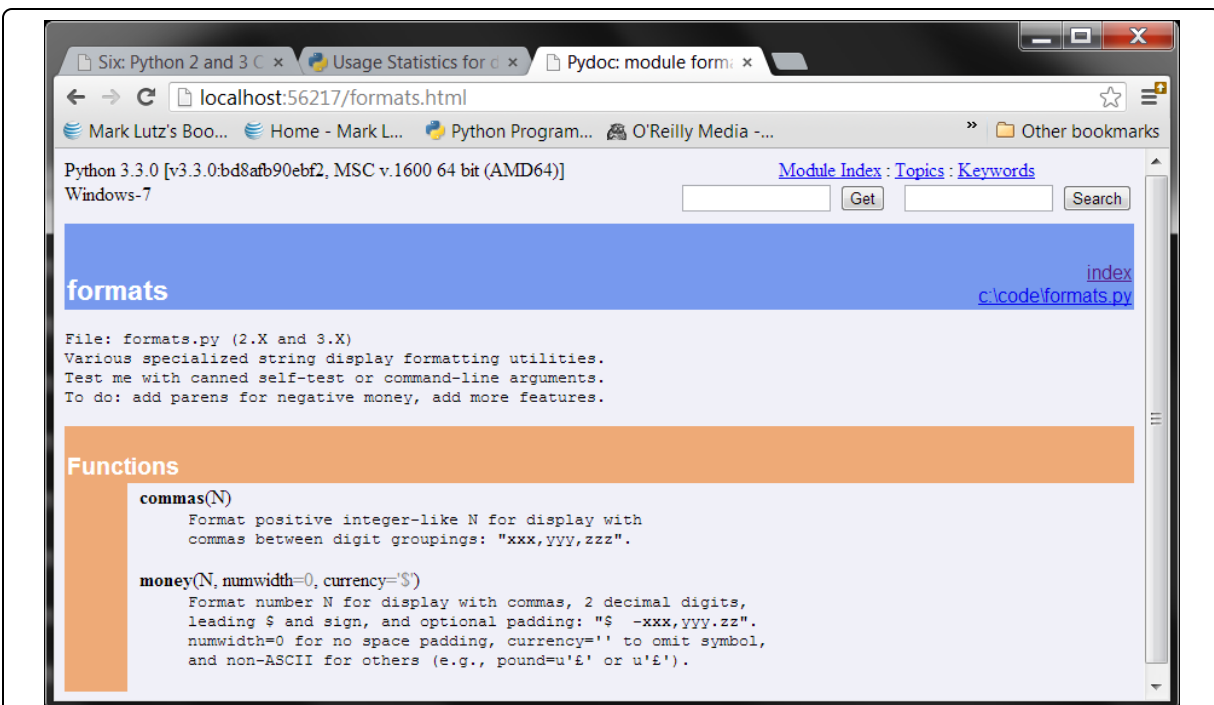
Figure 25-2. PyDoc's view of formats.py obtained by running a "py -3 -m pydoc -b" command line in 3.2 and later and clicking on the index entry (see Chapter 15 )
