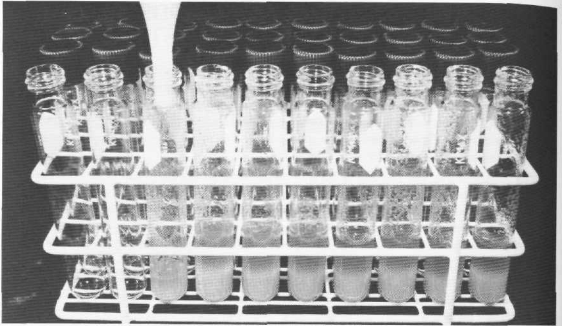
Figure 41 Filling test tubes with liquid agar media prior to sterilization in a pressure cooker.
