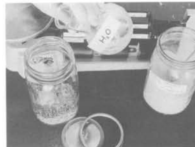
fig. 25: 150 milliliters of water are added.
