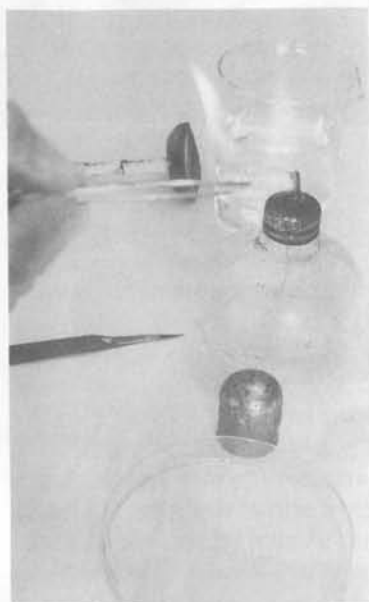
fig. 2: Sterilizing the slide.
