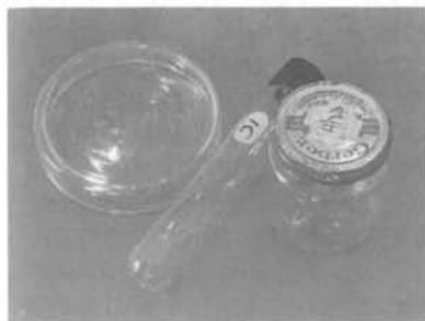
fig. 11: Three containers suitable for agar culture.
