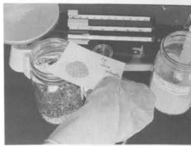
fig. 24: Two grams of powdered oyster shell (CaCO 3 ) are added.
