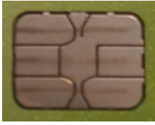
Figure 17.2: Smartcard integrated circuit chip shown from smartcard-enabled credit card
