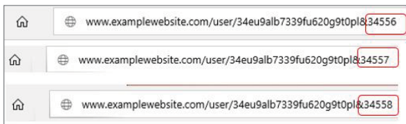
Figure 6.2: Example of sequentially incrementing session IDs located in a URL
