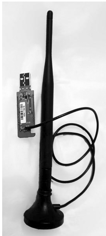
Figure 8.7 Bluetooth adapter with hacked connector and antenna.
