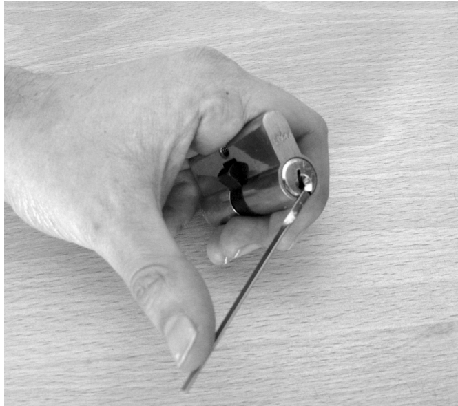
Figure 5.12 Lock with torque wrench inserted.
