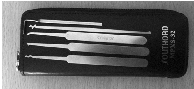
Figure 8.11 A pick set for opening pin tumbler locks.
