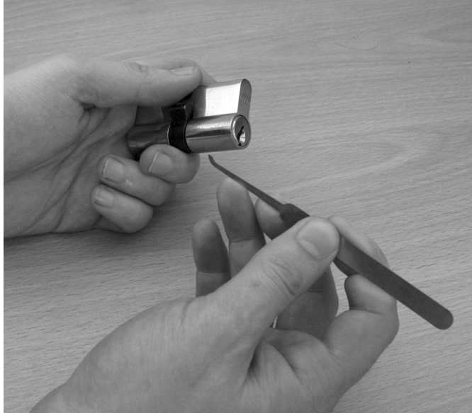
Figure 5.13 The lifter pick is used to set the pins.
